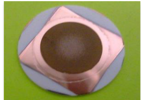
Monolithic Protected Lithium Cassette Anode Embedded on Ceramic Solid Electrolyte
